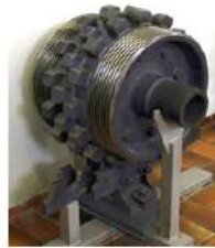
Figure 9: ABT Rack-and-Pinion System
